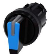
Selector switch, illuminable, 22 mm, round, plastic, blue, selector switch, short, 3 switch positions I-O-II, latching, actuating angle 2x45°, 10:30h/12h/13:30h, with laser labeling, upper case and lower case, always upper case at the beginning of the word
