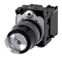
RONIS key-operated switch, 22 mm, round, plastic with metal front ring, lock number SB30, with 2 keys, 2 switch positions O-I, latching, actuating angle 90°, 10:30h/13:30h, key removal O+I, with holder, 1 NO, screw terminal, possible special locks: SB31, 421, 455, with laser labeling, upper case
