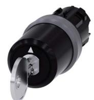
key-operated switch Siemens, 22 mm, round, plastic with metal front ring, lock number SSG10, with 2 keys, 3 switch positions I-O-II, latching, actuating angle 2x45°, 10:30h/12h/13:30h, key removal I, with laser labeling, upper case and lower case, always upper case at beginning of line
