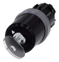
key-operated switch Siemens, 22 mm, round, plastic with metal front ring, lock number SSG10, with 2 keys, 2 switch positions O-I, latching, actuating angle 90°, 10:30h/13:30h, key removal O+I, with laser labeling, inscription or symbol customer-specific selection with SIRIUS ACT configurator (CIN)
