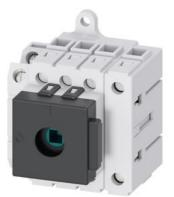
Load disconnector 3LD3, Iu 63 A Main switch 3-pole + N Rated operating capacity at AC-23 A at 400V 22.0 kW Installation in distribution boards, Basic switch without Knob-operated mechanism with auxiliary switch 10E + 1S
