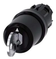
Key-operated switch IKON, 22 mm, round, plastic, lock number 360012K1, with 2 keys, 3 switch positions I-O-II, latching, actuating angle 2x45°, 10:30h/12h/13:30h, Key removal O Z=50-unit packaging
