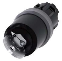
Key-operated switch IKON, 22 mm, round, plastic with metal front ring, lock number 360012K1, with 2 keys, 2 switch positions O<I, momentary contact type, Actuating angle 45°, 10:30h/12h, key removal O, with laser labeling, lower case
