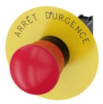
EMERGENCY STOP mushroom pushbutton, 22 mm, round, plastic, red, 40 mm, positive latching, acc. to EN ISO 13850, rotate-to-unlatch, with yellow backing plate, inscription: Arrêt d'urgence, with holder, 1 NC, screw terminal
