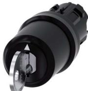
Key-operated switch IKON, 22 mm, round, plastic, lock number 360012K1, with 2 keys, 3 switch positions I-O<II, left latching, right momentary contact type, actuating angle  $2x45^{\circ}$ , 10:30h/12h/13:30h, Key removal O+I
