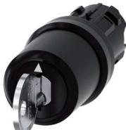
Key-operated switch IKON, 22 mm, round, plastic, lock number 360012K1, with 2 keys, 3 switch positions I>O<II, momentary contact type, actuating angle 2x45°, 10:30h/12h/13:30h, key removal O, with laser labeling, upper case
