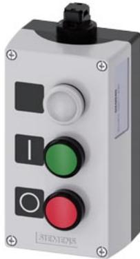
AS-Interface enclosure for command devices, 22 mm, round, Enclosure material plastic, enclosure top part gray, 3 control points plastic, Recess for labels, C=Indicator light clear, label without inscription, B=Pushbutton green, label: I, 1 NO, spring-type terminal, A=Pushbutton red, label: O, 1 NC, spring-type terminal, floor mounting, Insulation displacement system on top, Labels enclosed
