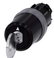
key-operated switch Siemens, 22 mm, round, plastic with metal front ring, special lock, with 2 keys, 3 switch positions I-O-II, latching, actuating angle 2x45°, 10:30h/12h/13:30h, key removal O+I
