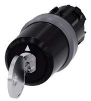
key-operated switch Siemens, 22 mm, round, plastic with metal front ring, lock number SSG10, with 2 keys, 3 switch positions I-O<II, left latching, momentary contact type on the right, actuating angle  $2x45^{\circ}$ , 10:30h/12h/13:30h, key removal O Z=50-unit packaging
