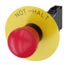
EMERGENCY STOP mushroom-type actuator, 22 mm, round, plastic, red, 40 mm, positive latching, according to EN ISO 13850, pull-to-unlatch mechanism, with yellow backing plate, inscription: NOT-HALT, with holder, 1 NO+1 NC, screw terminal
