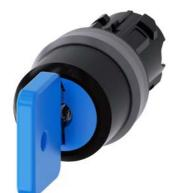
Key-operated switch O.M.R, 22 mm, round, plastic with metal front ring, lock number 73038, blue, with 2 keys, 3 switch positions I-O-II, latching, actuating angle 2x45°, 10:30h/12h/13:30h, Key removal I+O+II, with laser labeling, upper case and lower case, always upper case at beginning of line
