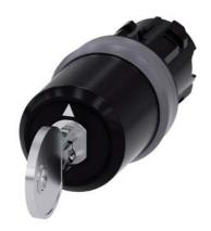
Key-operated switch BKS, 22 mm, round, plastic with metal front ring, lock number S1, with 2 keys, 3 switch positions I>O<II, momentary contact on the left, latching on the right, actuating angle  $2x45^{\circ}$ , 10:30h/12h/13:30h, key removal O, with laser labeling, upper case and lower case,
