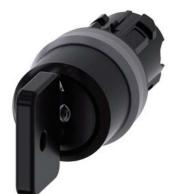
Key-operated switch O.M.R, 22 mm, round, plastic with metal front ring, lock number 73034, black, with 2 keys, 3 switch positions I-O-II, latching, actuating angle 2x45°, 10:30h/12h/13:30h, Key removal O
