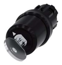
Key-operated switch BKS, 22 mm, round, plastic, lock No. E9 (VW), without key, 2 switch positions O-I, latching, actuating angle  $90^\circ$ , 10:30h/13:30h, key removal O, with laser labeling, upper case and lower case, always upper case at beginning of line
