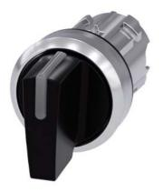
Illuminable selector switch, 22 mm, round, metal shiny, black, Selector switch short, 3 switch positions I>O<II, momentary contact type, actuating angle 2x45°, 10:30 /12 /13:30, Z=50-unit packaging
