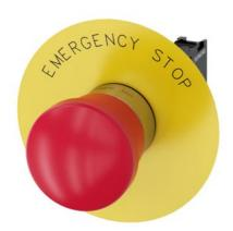
EMERGENCY STOP mushroom pushbutton, 22 mm, round, metal, shiny, red, 40 mm, positive latching, acc. to EN ISO 13850, pull-to-unlatch mechanism, with yellow backing plate, inscription: EMERGENCY STOP, with holder, 1 NC, screw terminal, Z=20-unit packaging
