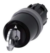
Key-operated switch IKON, 22 mm, round, plastic with metal front ring, lock number 360012K1, with 2 keys, 3 switch positions I-O<II, left latching, right momentary contact type, actuating angle  $2x45^{\circ}$ , 10:30h/12h/13:30h, key removal O+I, with laser labeling, upper case
