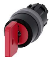
Key-operated switch O.M.R, 22 mm, round, plastic with metal front ring, lock number 73037, red, with 2 keys, 3 switch positions I-O-II, latching, actuating angle 2x45°, 10:30h/12h/13:30h, Key removal O+I
