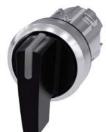
Illuminable selector switch, 22 mm, round, metal shiny, black, Selector switch long, 3 switch positions I>O<II, momentary contact on the left, latching on the right, actuating angle 2x45°, 10:30 /12 /13:30, Z=50-unit packaging
