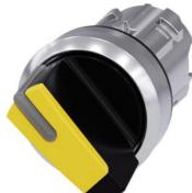
Illuminable selector switch, 22 mm, round, metal shiny, yellow, Selector switch short, 2 switch positions O-I, latching, actuating angle  $90^{\circ}$ , 10:30h/13:30h
