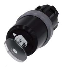
Key-operated switch BKS, 22 mm, round, plastic with metal front ring, Lock No. E7 (VW), without key, 2 switch positions O-I, latching, actuating angle  $90^\circ$ , 10:30h/13:30h, key removal O+I, with laser labeling, upper case and lower case, always upper case at the beginning of the word
