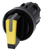
Selector switch, illuminable, 22 mm, round, plastic, yellow, selector switch, short, 3 switch positions I>O<II, momentary contact type, actuating angle 2x45°, 10:30h/12h/13:30h, with laser labeling, upper case and lower case, always upper case at the beginning of the word
