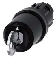
Key-operated switch IKON, 22 mm, round, plastic, lock number 360012K1, with 2 keys, 3 switch positions I-O<II, left latching, right momentary contact type, actuating angle 2x45°, 10:30h/12h/13:30h, key removal O+I, with laser labeling, lower case
