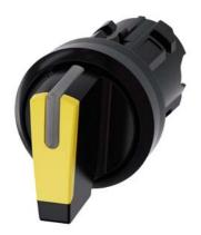
Selector switch, illuminable, 22 mm, round, plastic, yellow, selector switch, short, 3 switch positions I-O<II, left latching, right momentary contact type, actuating angle  $2x45^{\circ}$ , 10:30h/12h/13:30h, with laser labeling, upper case
