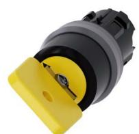
Key-operated switch O.M.R, 22 mm, round, plastic with metal front ring, lock number 73033, yellow, with 2 keys, 2 switch positions O<1, momentary contact type, Actuating angle 45°, 10:30h/12h, key removal O, with laser labeling, upper case and lower case, always upper case at the beginning of the word
