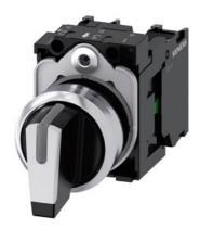
Selector switch, illuminable, 22 mm, round, metal, shiny, white, selector switch, short, 3 switch positions I-O-II, latching, actuating angle  $2x45^{\circ}$ , 10:30h/12h/13:30h, with holder, 1 NO, 1 NO, screw terminal, Z=20-unit packaging
