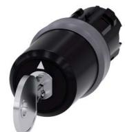
key-operated switch Siemens, 22 mm, round, plastic with metal front ring, lock number SSG10, with 2 keys, 3 switch positions I>O<II, momentary contact on the left, latching on the right, actuating angle  $2x45^{\circ}$ , 10:30h/12h/13:30h, key removal II, with laser labeling, upper case
