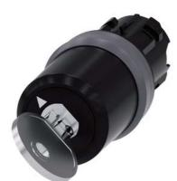
Key-operated switch BKS, 22 mm, round, plastic with metal front ring, lock number S1, with 2 keys, 2 switch positions O-I, latching, actuating angle 90°, 10:30h/13:30h, key removal I, Z=50-unit packaging
