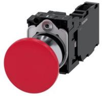
Mushroom pushbutton, 22 mm, round, metal, shiny, red, 40mm, latching, pull-to-unlatch mechanism, with holder, 1 NO+1 NC, screw terminal, with laser labeling, upper case and lower case, always upper case at beginning of line
