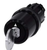
key-operated switch Siemens, 22 mm, round, plastic, special lock, with 2 keys, 3 switch positions I-O-II, latching, actuating angle 2x45°, 10:30h/12h/13:30h, key removal I+II
