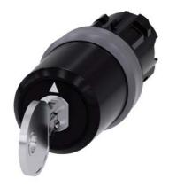
key-operated switch Siemens, 22 mm, round, plastic with metal front ring, lock number SSG10, with 2 keys, 3 switch positions I-O<II, left latching, momentary contact type on the right, actuating angle  $2x45^\circ$ , 10:30h/12h/13:30h, key removal I
