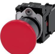
Mushroom pushbutton, 22 mm, round, plastic with metal front ring, red, 40mm, latching, pull-to-unlatch mechanism, with holder, 1 NC, screw terminal, with laser labeling, upper case and lower case, always upper case at beginning of line
