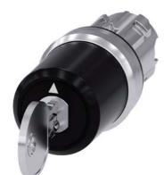
Key-operated switch BKS, 22 mm, round, metal, shiny, lock number S1, with 2 keys, 3 switch positions I>O<II, momentary contact type, actuating angle 2x45°, 10:30h/12h/13:30h, key removal O, with laser labeling, upper case and lower case, always upper case at beginning of line
