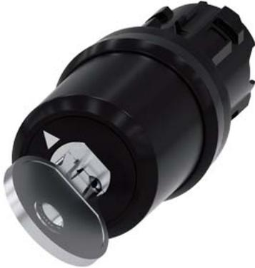
Key-operated switch BKS, 22 mm, round, plastic, lock No. E9 (VW), without key, 2 switch positions O-I, latching, actuating angle 90°, 10:30h/13:30h, key removal O+I, with laser labeling, upper case and lower case, always upper case at beginning of line
