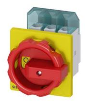
SENTRON, Switch disconnector 3LD, emergency switching-off switch, 3- pole, lu: 32 A, operating power / at AC-23 A 400 V: 11.5 kW, front-mounted, rotary operating mechanism, Red / yellow, 4-hole mounting of the handle
