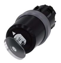
Key-operated switch BKS, 22 mm, round, plastic with metal front ring, lock number S1, with 2 keys, 2 switch positions O-I, latching, actuating angle  $90^\circ,$  10:30h/13:30h, key removal O+I, with laser labeling, upper case and lower case, always upper case at the beginning of the word
