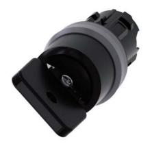
Key-operated switch O.M.R, 22 mm, round, plastic with metal front ring, lock number 73034, black, with 2 keys, 2 switch positions O-I, latching, actuating angle 90°, 10:30h/13:30h, key removal O+I, with laser labeling, upper case
