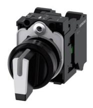
Selector switch, illuminable, 22 mm, round, plastic, white, selector switch, short, 3 switch positions I-O-II, latching, 10:30h/12h/13:30h, with holder, 1 NO, 1 NO, Spring-type terminal
