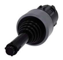
Coordinate switch, 22 mm, round, plastic with metal front ring, black, 2 switch positions, horizontal latching, with mechanical interlocking, with laser labeling, inscription or symbol, Customer-specific selection with SIRIUS ACT configurator (CIN)
