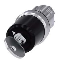
key-operated switch Siemens, 22 mm, round, metal, shiny, lock no. STGH10, with 2 keys, 2 switch positions O<I, momentary contact type, actuating angle 45°, 10:30h/12h, key removal O, with laser labeling, upper case and lower case, always upper case at the beginning of the word
