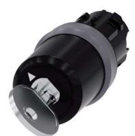
key-operated switch Siemens, 22 mm, round, plastic with metal front ring, special lock, with 2 keys, 2 switch positions O-I, latching, actuating angle 90°, 10:30h/13:30h, key removal I
