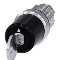
key-operated switch Siemens, 22 mm, round, metal, shiny, lock no. STGH10, with 2 keys, 3 switch positions I>O<II, momentary contact type, actuating angle 2x45°, 10:30h/12h/13:30h, key removal O, with laser labeling, upper case and lower case, always upper case at beginning of line
