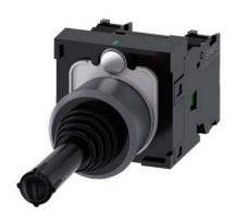
Coordinate switch, 22 mm, round, plastic with metal front ring, black, 2 switch positions, horizontal, momentary contact type, without mechanical interlocking in O position, with holder, 1 NO, 1 NO, screw terminal, with laser labeling, inscription or symbol Customer-specific selection with SIRIUS ACT configurator (CIN)
