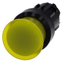
Illuminated mushroom pushbutton, 22 mm, round, plastic, yellow, 30 mm, momentary contact type, with laser labeling, upper case  $\,$
