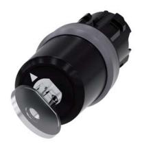
Key-operated switch BKS, 22 mm, round, plastic with metal front ring, special lock, with 2 keys, 2 switch positions O<I, momentary contact type, actuating angle 45°, 10:30h/12h, key removal O, Note: BKS locking systems E1 - E25 supplied without key
