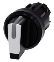
Selector switch, illuminable, 22 mm, round, plastic, white, selector switch, short, 3 switch positions I>O<II, momentary contact on the left, latching on the right, actuating angle  $2x45^{\circ}$ , 10:30h/12h/13:30h, with laser labeling, upper case
